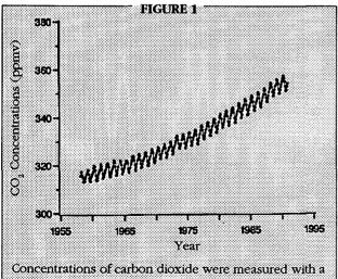
Concentrations of carbon dioxide were measured with a continuously recording nondispersive infrared gas analyzer at Mauna Loa Observatory, Hawaii. The dots indicate average monthly concentrations.
