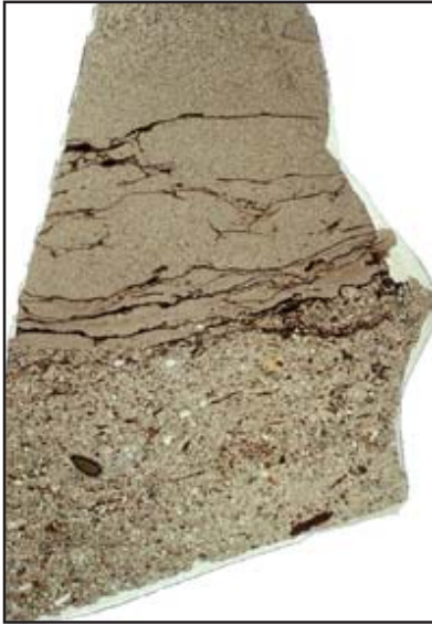
Figure 14. A microslide of a thin section from an organic level in the Cache Creek area. The wavy dark horizontal lines are cross-sections of deciduous leaves. Note the following features: a) clean ash or sand between the leaves; b) sudden change in grain size between the upper and lower halves of the organic level; and c) different types of organic debris in the fine and coarse sediments.
